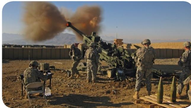
**Figura 1 – Obus 155 mm M777 *Lightweight* (Rebocado)**
