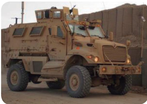
Figura 11 – Viatura Mine-Resistant Ambush Protected (MRAP) modelo MaxxPro
