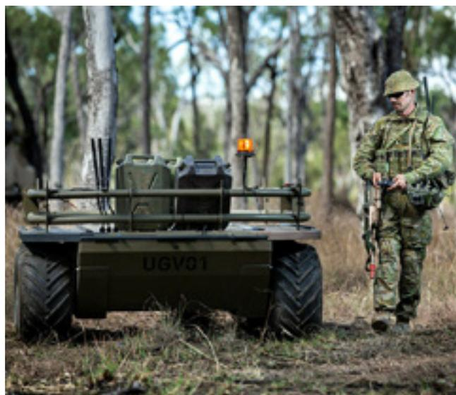
Figura 05: Mission adaptable platform System (MAPS) STNT – Austrália. Fonte: (Mission Adaptable Platform System (MAPS) UGV, 2021)
