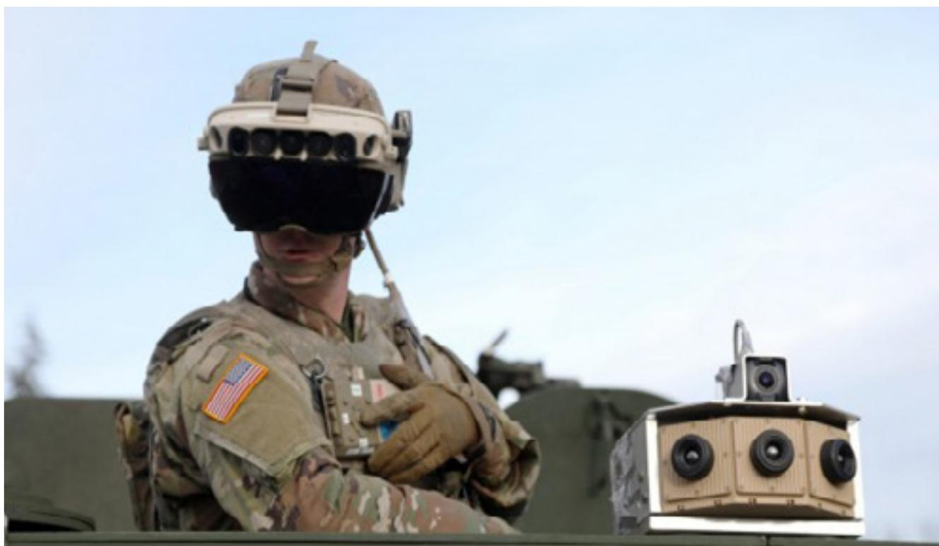
Figura 04: US Army Integrated Visual Augmentation System (IVAS) montado numa VBR Stryker.
