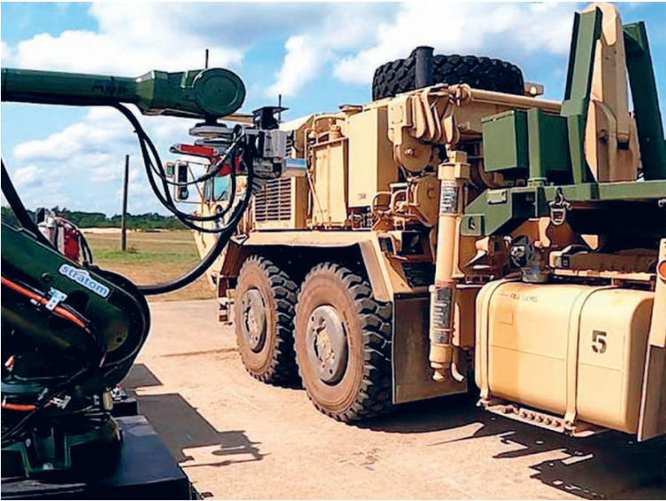
Fig. 3 - RAPID™ — Stratom's Autonomous Refueling, Recharging and Liquid Transfer System
